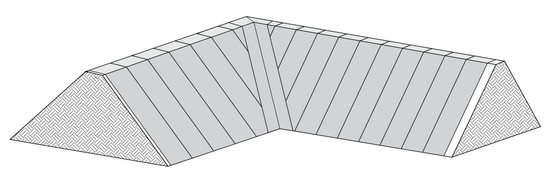
Detail A — CC Hydro Bund Corner Deployment Plan
