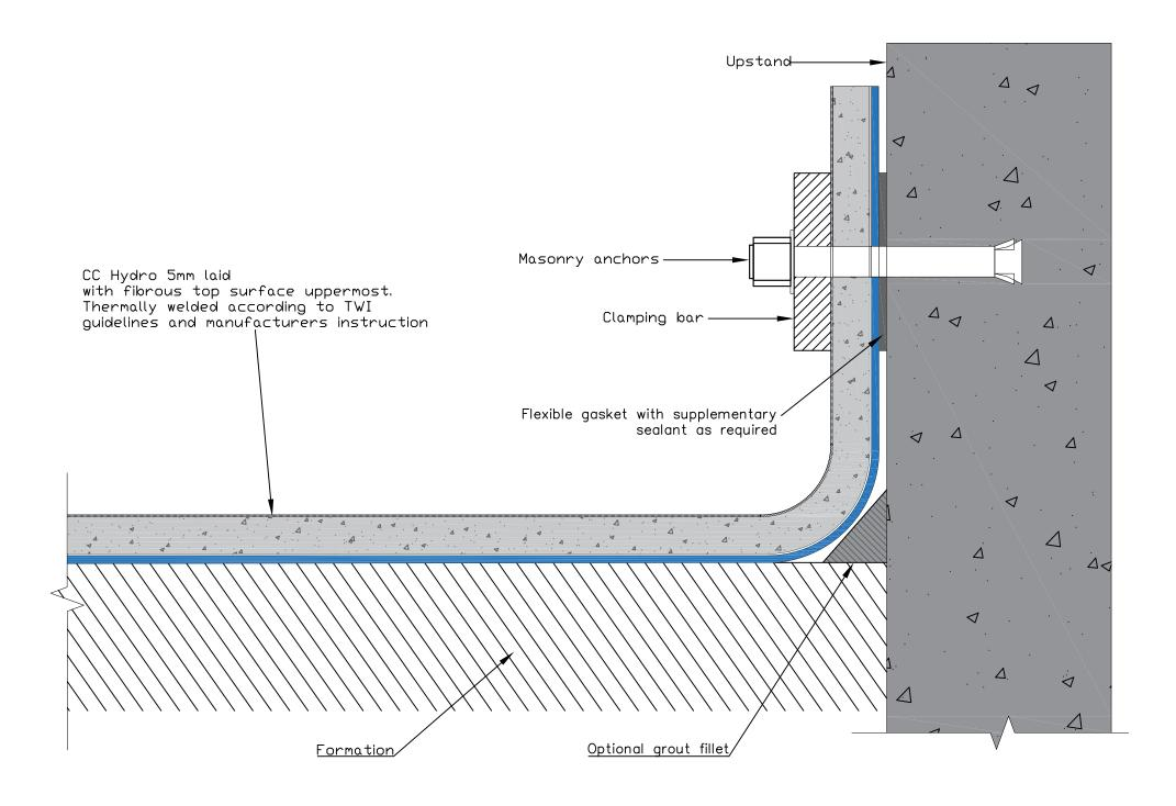
Detail A - CC Hydro to Concrete Wall Termination
